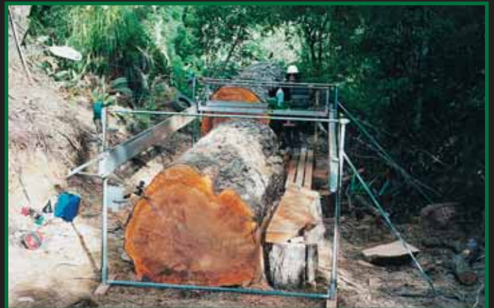
ADJUSTABLE FRAMEWORK FOR PARALLEL TO GRAIN CUTTING
